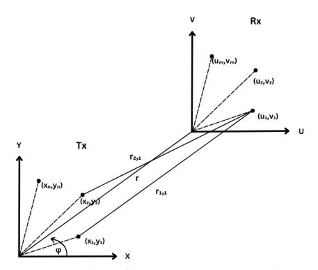
Figure 3. Schematic diagram of the MIMO antenna on XY and UV coordinate planes.
