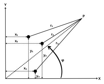
Figure 4. Schematic diagram of dipole placement in XY coordinate plane.
