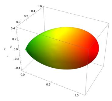
**Figure 7.** Three-dimensional view of the single beam formed at 30° when the transmitter antenna elements are half-wave dipoles.
