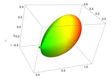
**Figure 10.** The same beam is shown at an angle for a better view of the side lobes. The side lobes have negligible energy.
