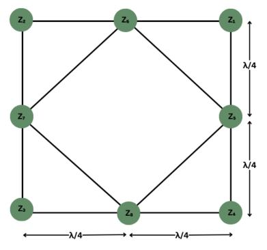
Figure 5. Proposed eight-element dipole antenna.
