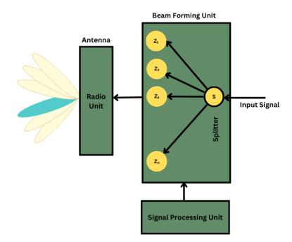
Figure 1. Transmitter antenna of the proposed MIMO system.
