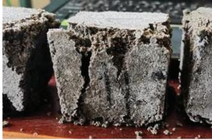
(b) Mortar with 5% of Polyester fibre Fig. 12. Post peak behaviour
