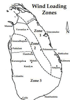
Figure 1 Wind Zone of Sri Lanka (Lewangamage & Jayasinghe 2012)
