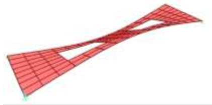
Figure 12: Higher order flexural vibration mode of skybridge (frequency – 25.5 Hz)
