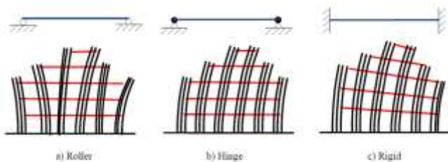
Figure 1: Different connection configuration and structural behaviour.
