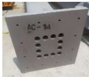
Figure 20: Base plate for CFST column.
