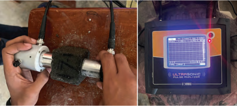
Figure 4. The measurement of UPV of mortar cube and measuring instrument.
