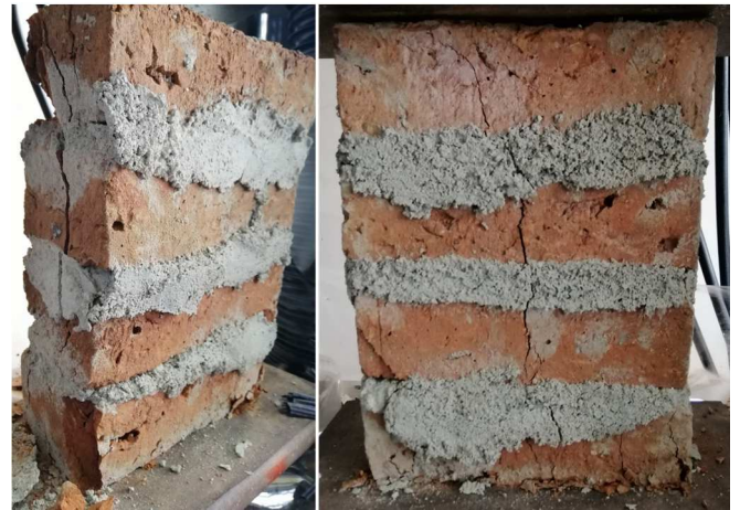
Fig. 8. Failure pattern observed in masonry prisms
