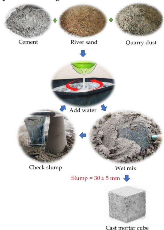
Figure 4 Cube casting procedure
