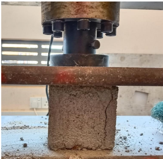
Figure 5 Testing of cubes for compression
