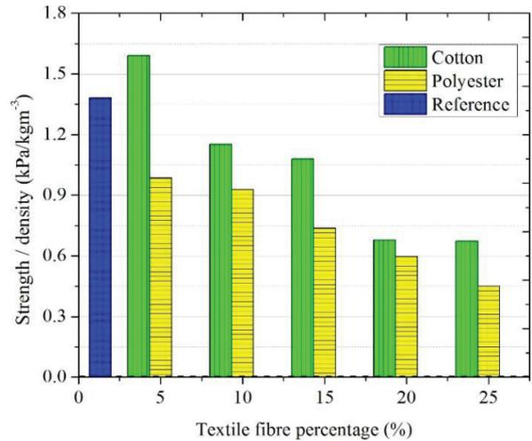
Fig. 11. Variation of strength/density at 28<sup>th</sup> day under wet conditions.
