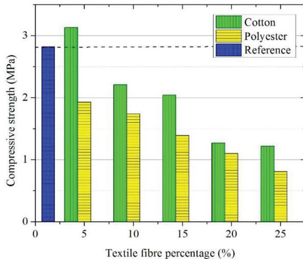
Fig. 10. 28<sup>th</sup> day compressive strength under wet conditions
