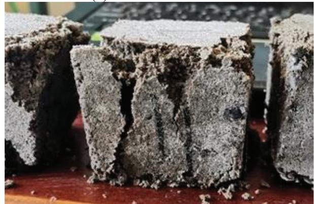
(b) Mortar with 5% of Polyester fibre
