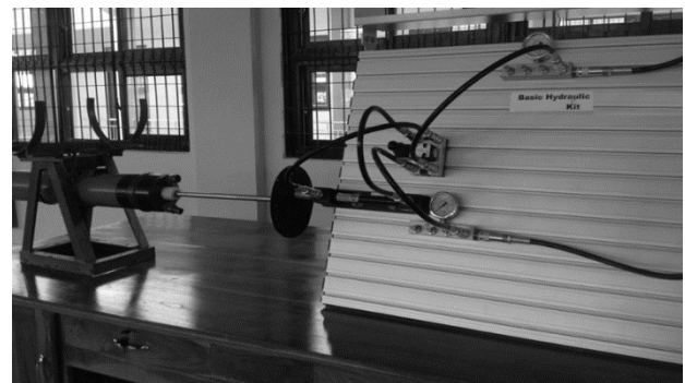
Figure 7 - Experimental Setup to Obtain Applied Force vs Developed Pressure Characteristics.
