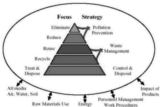
Fig 1. Integrated approach of Cleaner Production [5]
