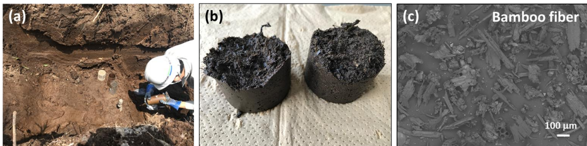
Figure 1: (a) Sampling peat soil, (b) appearance of peat soil and level of decomposition (c) SEM image of discrete bamboo fibers
