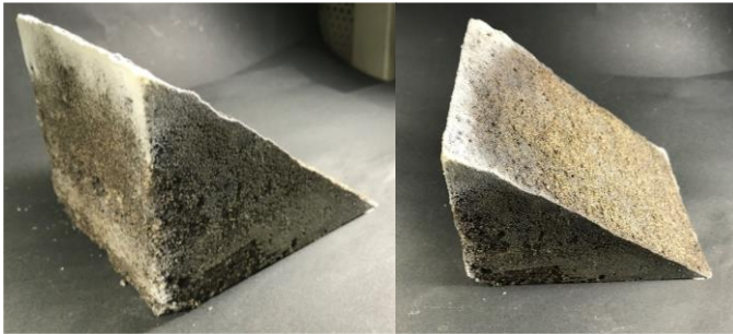
Fig. 3. Profile of the bio-cemented slope before flushing the salts and uncemented soil particles.
