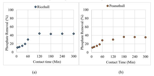
Figure 3: Phosphate Removal from Rice mill effluent by waste derived bio sorbents for different contact time (agitation speed: 150 rpm, Particle size < 1 mm), (a) Rice hull (3 g/L) (b) Peanut hull (4 g/L).
