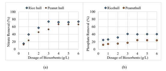
Figure 1: Removal of Nutrients from Rice mill wastewater by Rice hull and Peanut hull [dosage 0-7 g/L; contact time of 4 hours at 150 rpm; Particle size <1 mm] (a) Nitrate Removal (b) Phosphate Removal.
