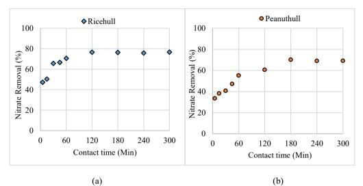
Figure 2: Nitrate Removal from Rice mill effluent by the biosorbents for different contact time (shaking: 150 rpm, Particle size < 1 mm), (a) Rice hull (3 g/L) (b) Peanut hull (4g/L).
