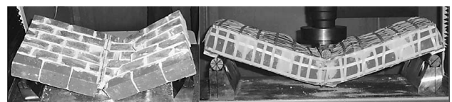
Fig. 8 Failure patterns of brick masonry wallettes with and without retrofitting by PP-band mesh
