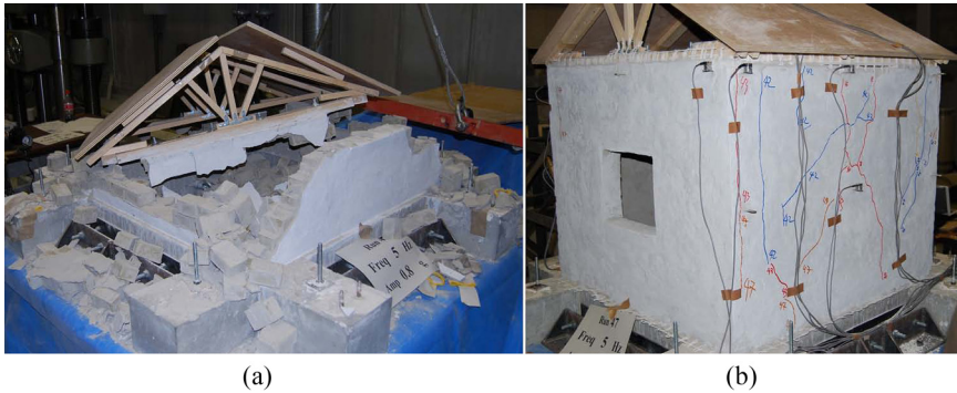
Figure 14. (a) The unretrofitted model, A-NR-P, and (b) the retrofitted model, A-RE-P, after Run 47.
