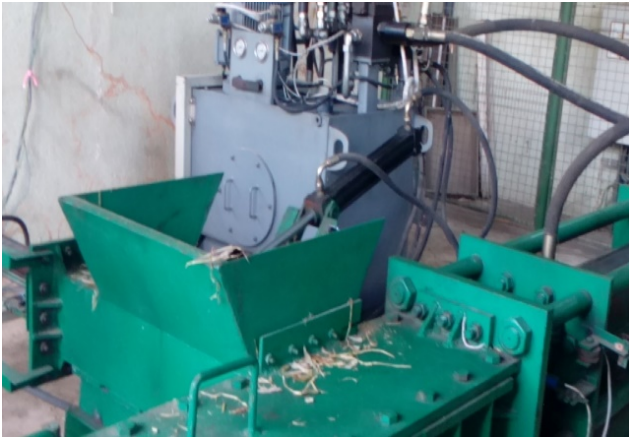
Figure 1: Compressed solid feed block making machine
