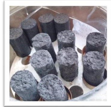
Fig. 1 Air curing of UCS samples
