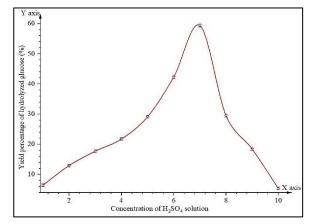
Figure 3: The yield percentage of hydrolyzed glucose from  $1.0 \times 10^4$  ppm of extracted cellulose with the constant agitating speed (400 rpm) for 4 hours and maintained at 30 °C for the various concentration of H<sub>2</sub>SO<sub>4</sub> solution.
