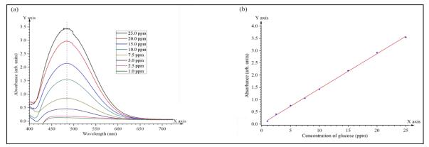
Figure 1: (a) The absorbance spectra of various concentration of standard glucose solutions in the presence of DNS reagent within the wavelength range 400 nm - 720 nm and (b) The standard calibration curve for the standard glucose solution at the optimum wavelength 484.0 nm.
