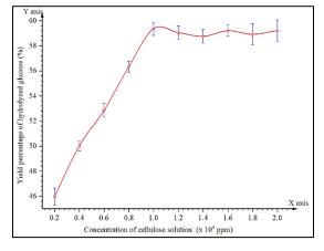
Figure 2: The yield percentage of hydrolyzed glucose as a function of extracted cellulose from PFH fibers with a constant agitating speed (400 rpm) and concentration of  $H_2SO_4$  (7.0 mol L<sup>-1</sup>) for 4 hours at 30 °C.
