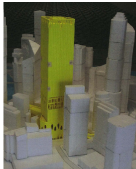
Figure 2a: Sample of wind tunnel test Model arrangement
