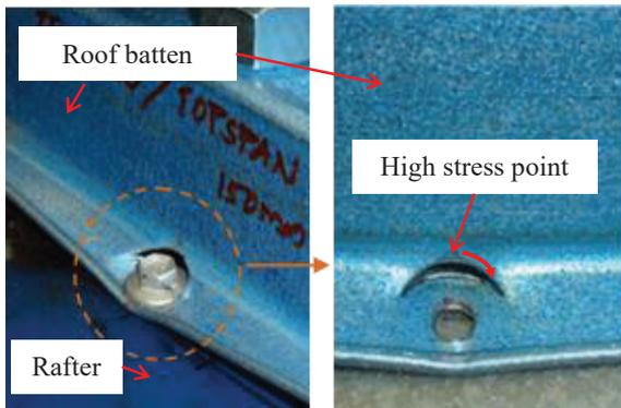
Fig. 2. Pull-through Failures of Steel Roof Batten
