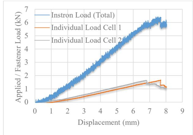
Fig. 6. Applied/Fastener Load versus Displacement Curves from Two-span Batten Tests Conducted using 0.48 mm Roof Battens and 10g Screw Connections.
