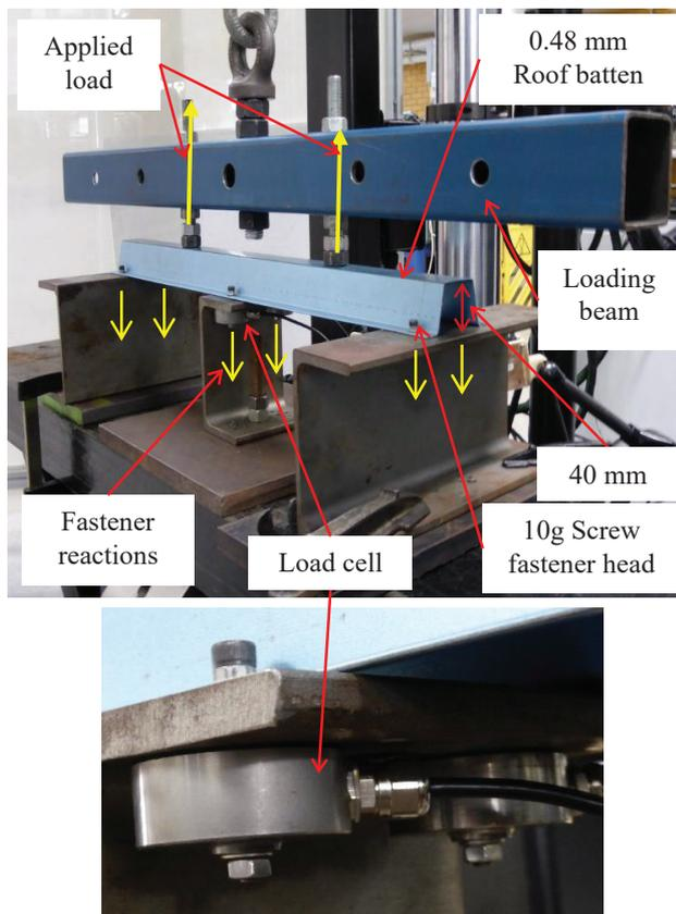
Fig. 3. Two-span Roof Batten Test Set-up
