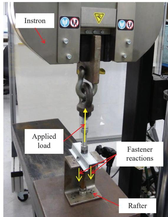
Fig. 4. Short Batten Test Set-up
