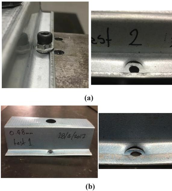
Fig. 5. Pull-through Failure Modes of (a) 0.42 mm Batten and (b) 0.48 mm Batten
