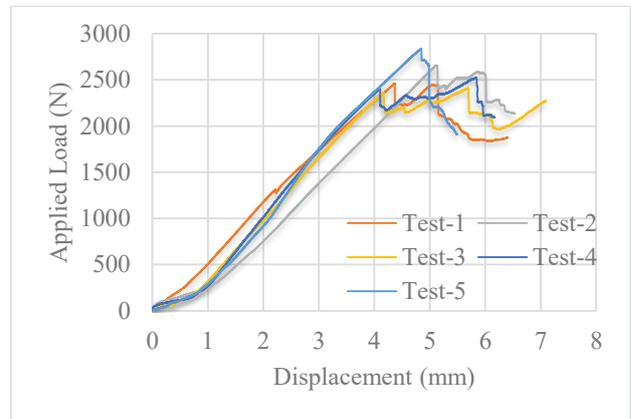
Fig. 7. Applied Load versus Displacement Curves from Short Batten Tests Undertaken using 0.42 mm Roof Battens and 10g Screw Connections.
