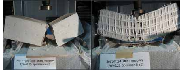
Figure 10 Failure Pattern of Stone Masonry Walette (Left: without Retrofitting, Right: with Retrofitting)
