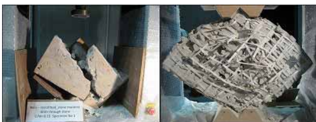
Figure 6 Failure Pattern of Stone Masonry Walette (Left: without Retrofitting, Right: with Retrofitting)
