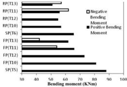
Figure 4. Comparison of maximum bending moment.
