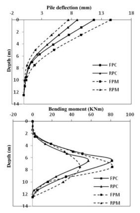
Figure 2. (a) Pile deflection and (b) Pile bending moment for Test 10.
