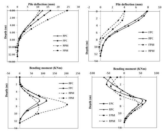
Figure 5. (a) Pile deflection and (b) Pile bending moment for Test 8.
