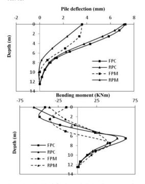
Figure 8. (a) Pile deflection and (b) bending moment for Test 13.
