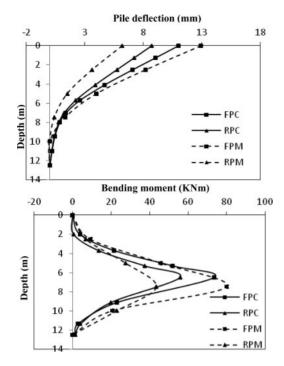
Figure 7. (a) Pile deflection and (b) bending moment for Test 12.
