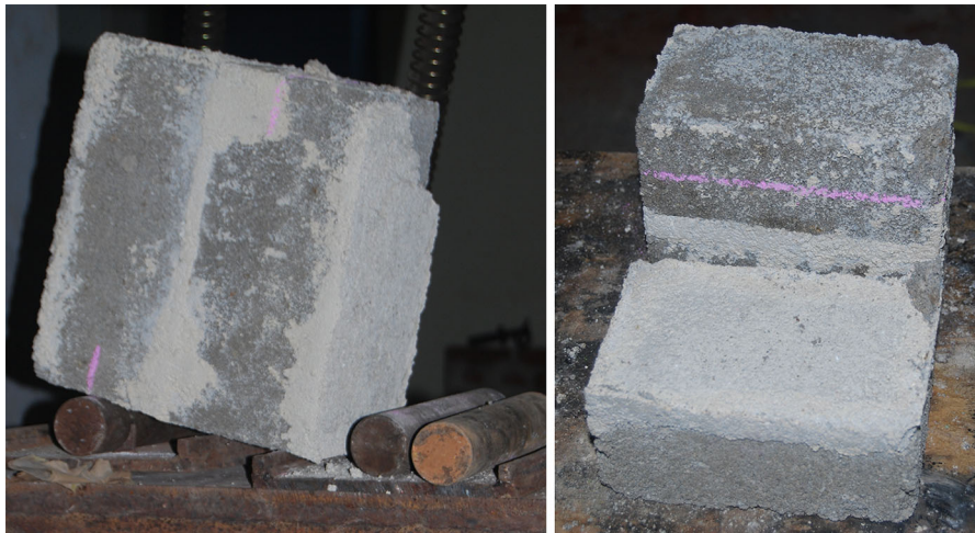
Fig. 5 Shear failure surface of cement block masonry
