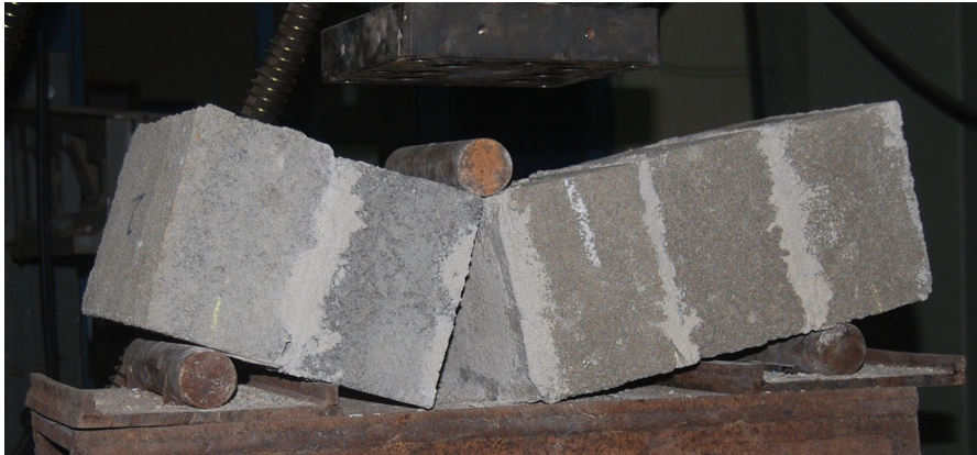
Fig. 7 Flexural bending failure surface of cement block masonry
