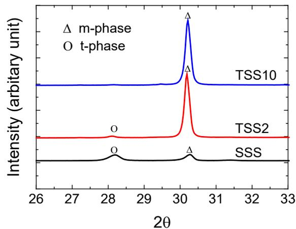
Fig. 2. XRD spectrum for 3Y-TZP samples sintered using SSS, TSS2 and TSS10 sintering profiles after 60 hours of ageing.
