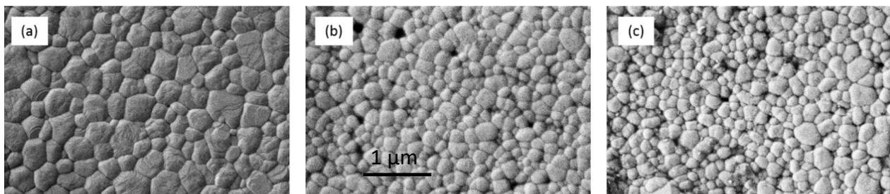
Fig. 1. FESEM images of (a) SSS, (b) TSS2 and (c) TSS10 samples.
