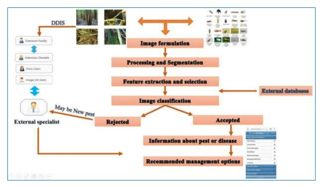
Fig. 1: Schematic representation of coupled DDIS and automated image processing for pest and disease detection
