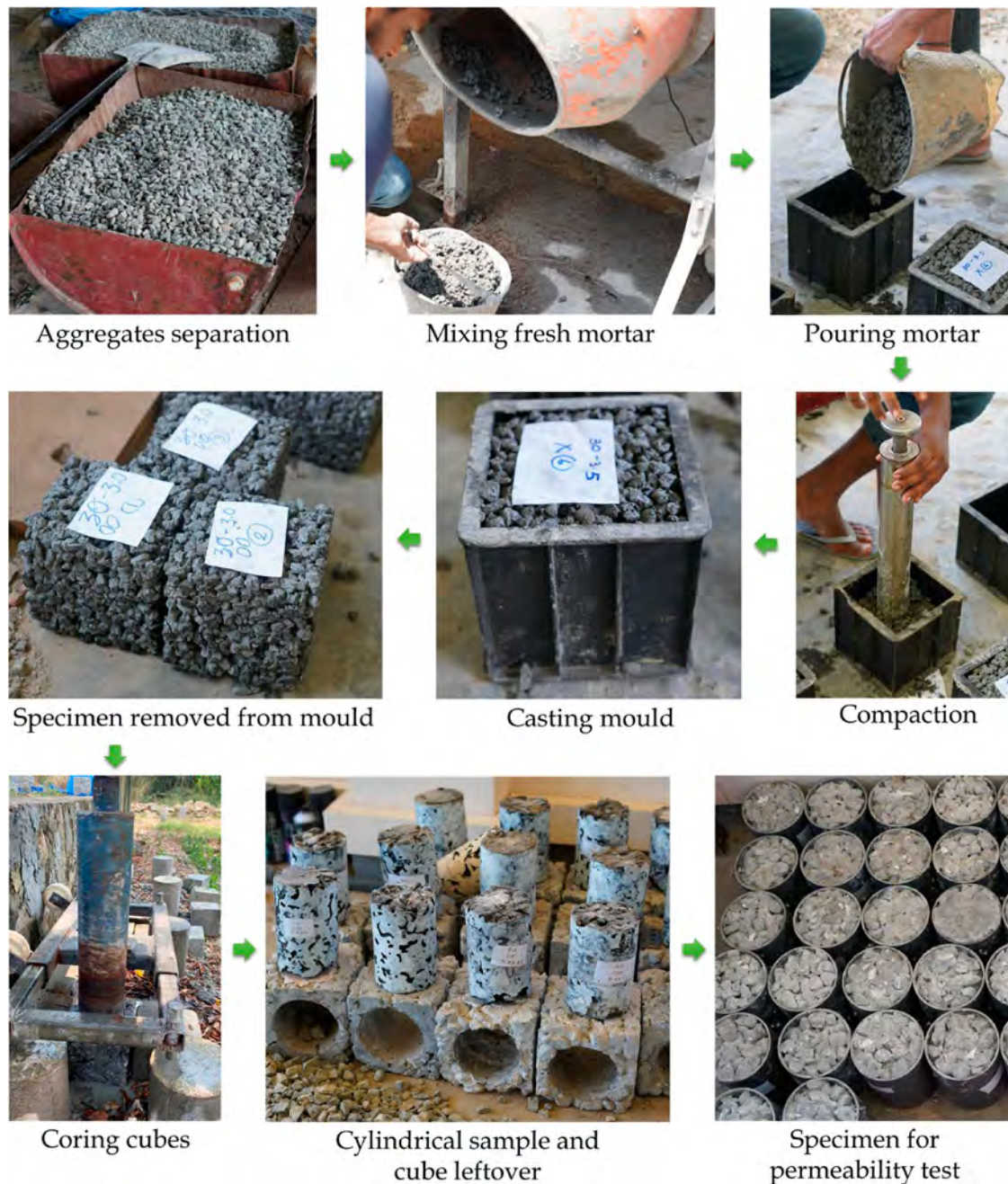
Figure 2. Pervious concrete cube preparation procedure.
