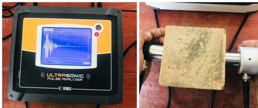
Fig. 4 UPV measurement equipment and setup
