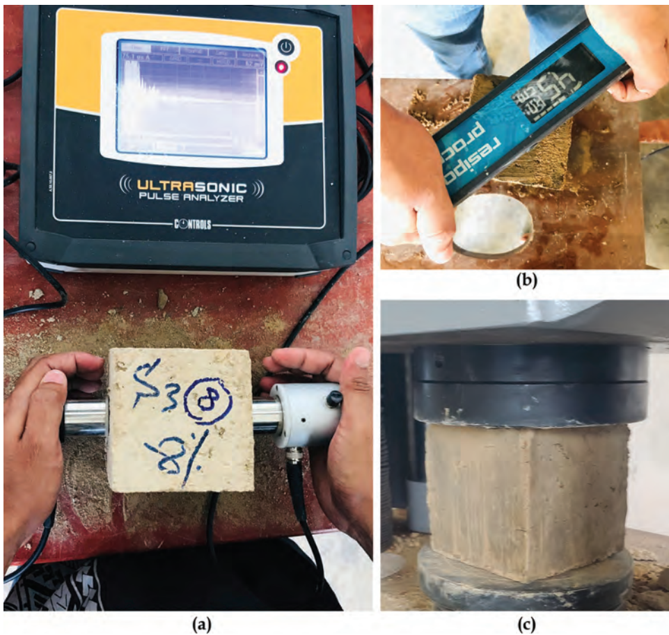
Figure 3. Testing setup (a) UPV, (b) ER, and (c) compression.
