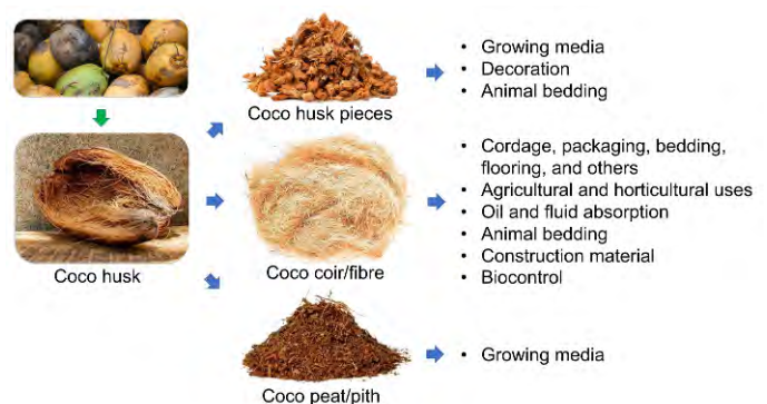
Fig 1. Derivation of by-products of the Coconut extraction process and its commercial use
