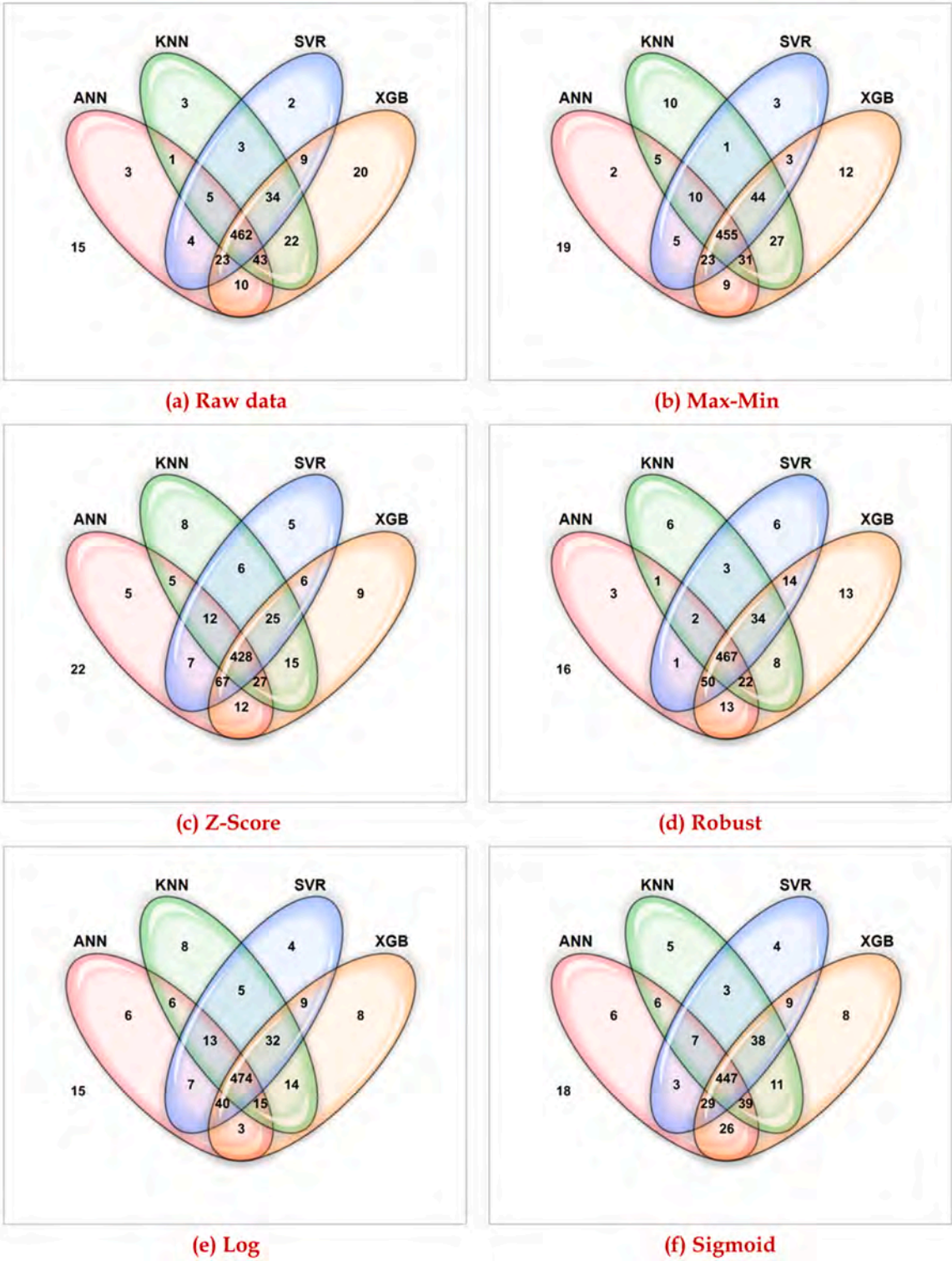
Fig. 13. Venn diagram for the number of data points with prediction error within 20 % of actual values. The areas where the ellipses overlap indicate the datapoints shared between the machine learning models, while the non-overlapping areas represent elements unique to each set.
