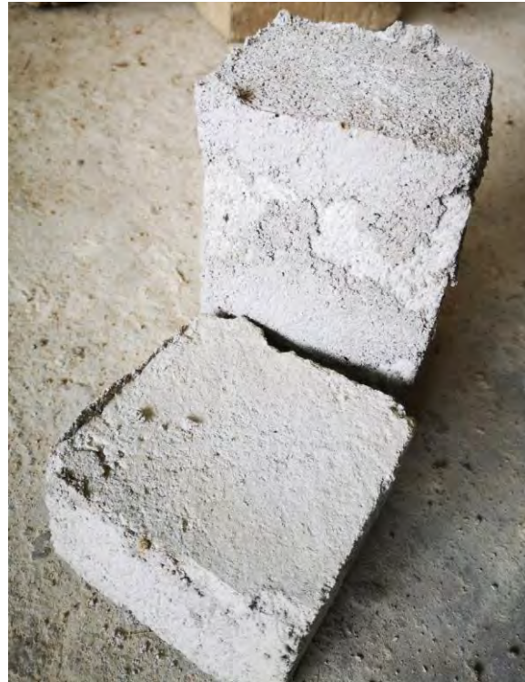
Fig. 7 - Failure pattern detected during shear tests
