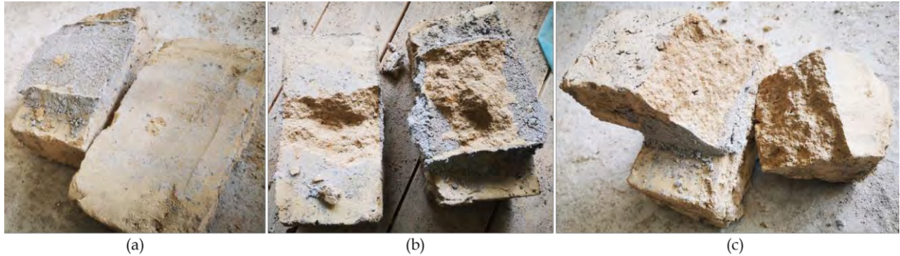
Fig. 9 - Failure patterns of the masonry wallet during bond failure (a) Type A; (b) Type B and; (c) Type C
