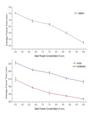
Figure 2: Fixture time variation with respect to seed powder concentration for different materials
