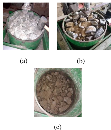
Fig. 3 Large scale direct shear test samples of (a) Fresh ballast; (b) Sand fouled ballast; (c) Clay fouled ballast
